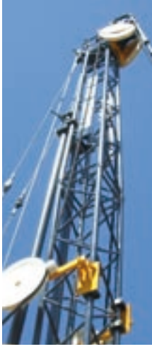
Hose sheave Ø 1.100 mm to a ground auger device
