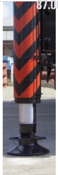
Polyamide float pads Ø 400 mm on a railway crane
